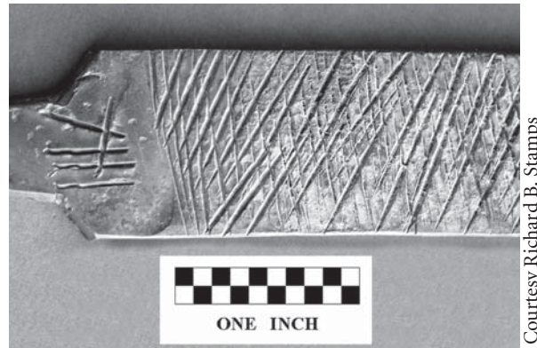
FIG. 11. The file’s cross-hatching. The cross-hatching departs significantly from a functional design. The cuts merely spread the metal rather than creating the curled-up pieces of metal composing the cutting edges. Also note the irregularities in spacing, depth, and angle.
