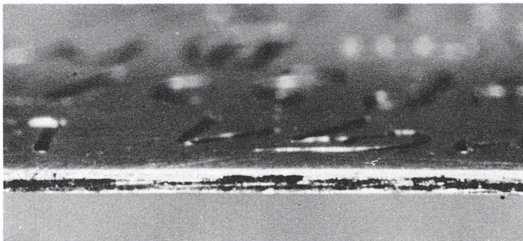
Figure 3. One edge of Plate 10 showing that it was filed to size. Note file marks running lengthwise on the edge.
